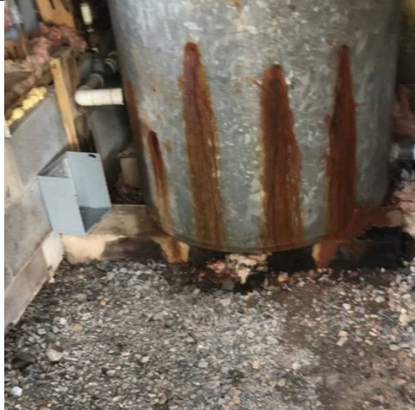
Holes in Tank Due to Rusting
