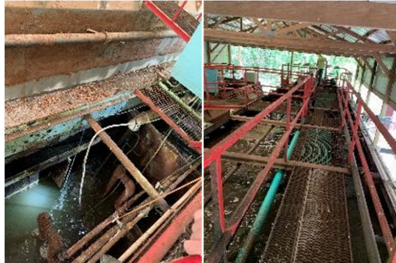
Severe corrosion and rust found throughout the plants.
