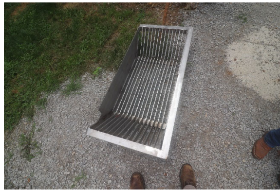
9 10 New bar screen pre-install
