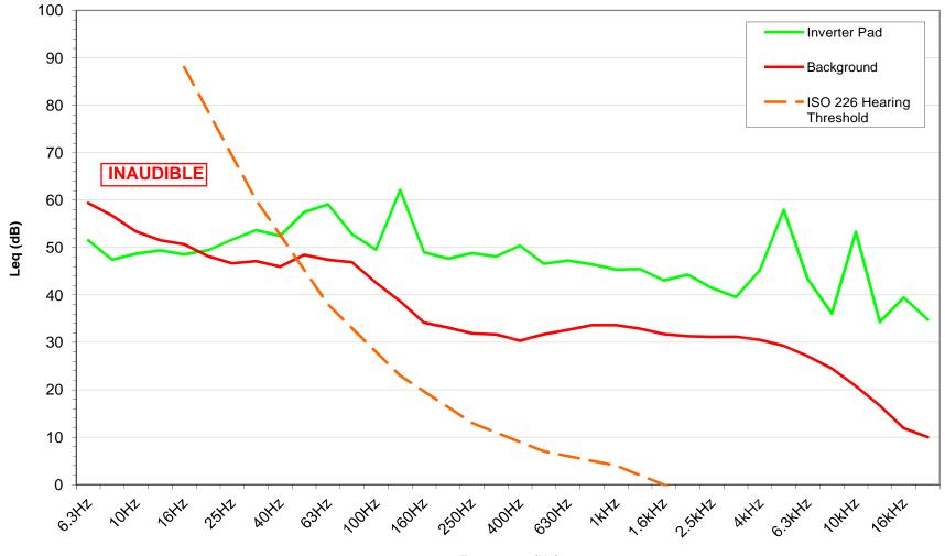
Figure 11. Frequency Spectrum of Sound Levels (Leq) at a Distance of 10 Feet from the Inverter Pad at Site #3
