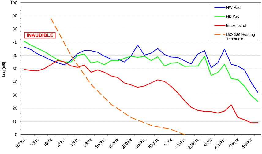
Figure 5. Frequency Spectrum of Sound Levels (Leq) at a Distance of 10 Feet from the Inverter Pads for Site #1
