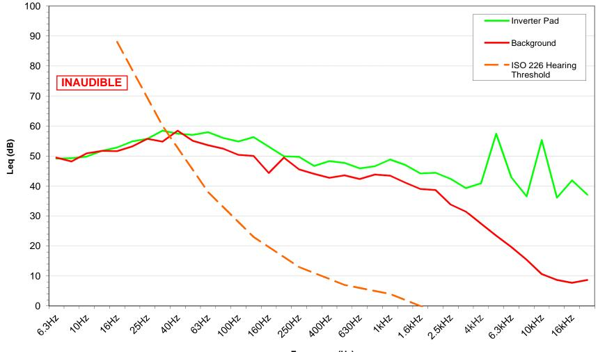
Figure 8. Frequency Spectrum of Sound Levels (Leq) at a Distance of 10 Feet from the Inverter Pad at Site #2
