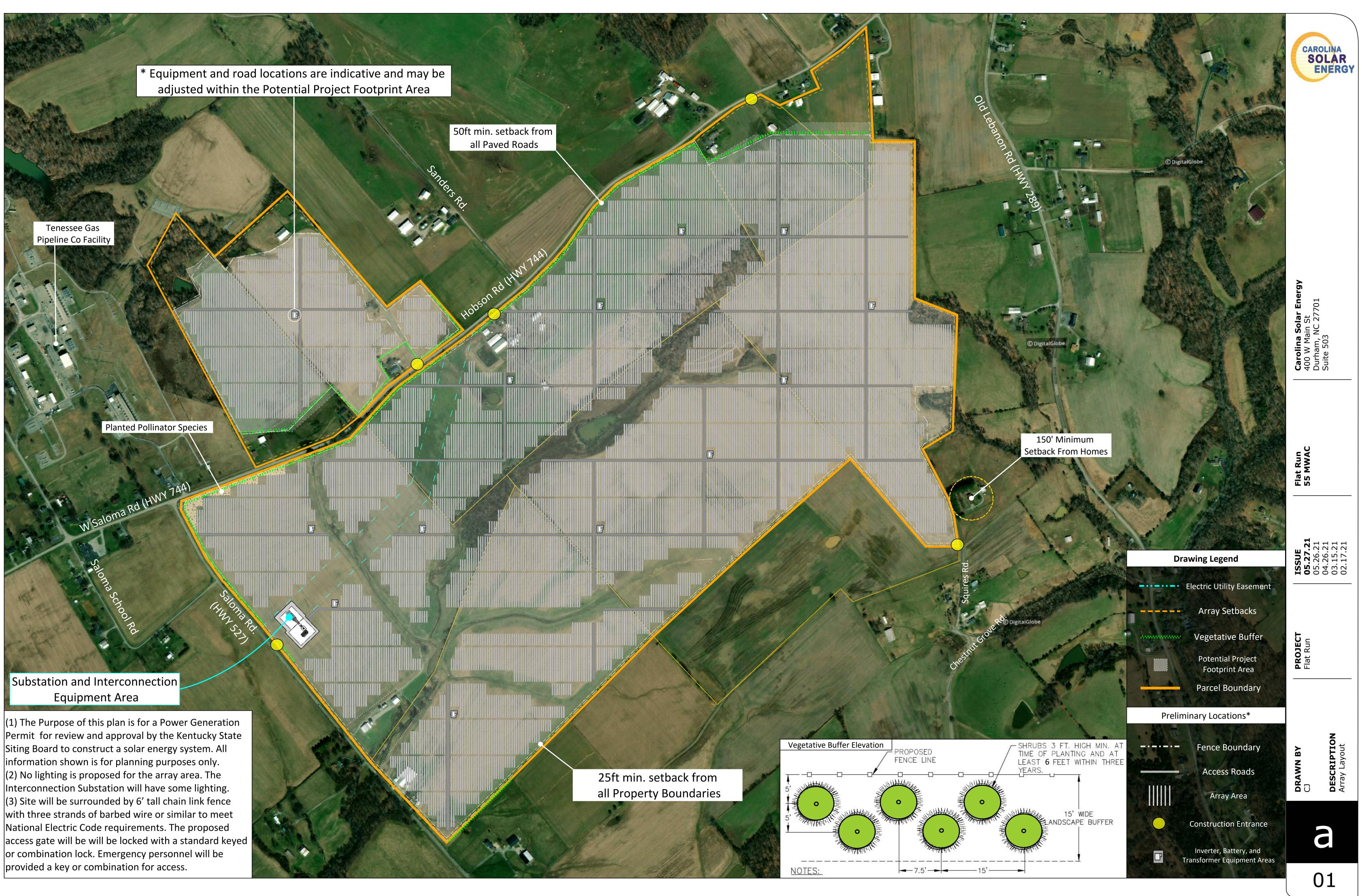
Siting Board to construct a solar energy system. All information shown is for planning purposes only. (2) No lighting is proposed for the array area. The Interconnection Substation will have some lighting. (3) Site will be surrounded by 6' tall chain link fence with three strands of barbed wire or similar to meet National Electric Code requirements. The proposed or combination lock. Emergency personnel will be provided a key or combination for access.
