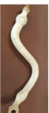
3/4" lead service line
