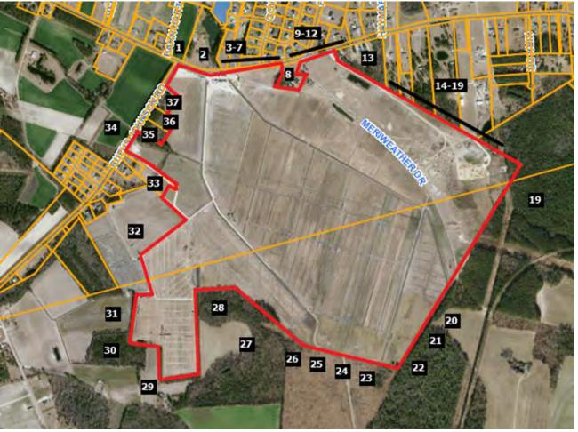
This project was built in 2017 and located on 413.99 acres for a 71 MW with the closest home at 135 feet from the closest solar panel with an average distance of 375 feet.
