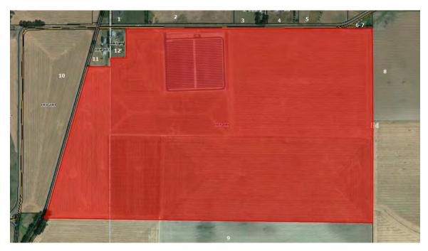
This solar farm has a 1.2 MW output and is located on a 186.60 acre tract using less than 10 of those acres. The project was built in 2011.
