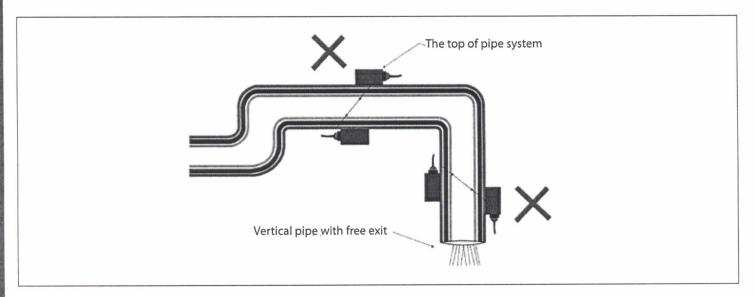
• For the open pipe or half full pipe, the transducers should be installed at the bottom of U pipe.
