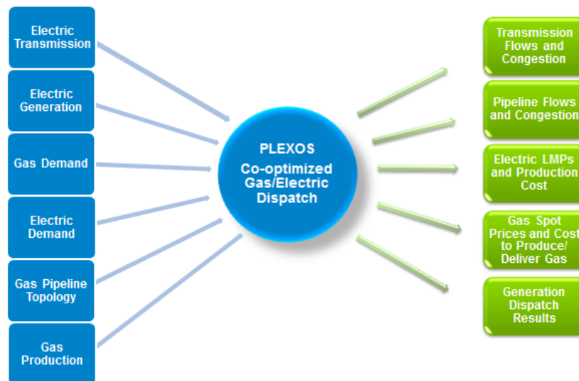
Figure 6.3-1: High-level inputs and outputs for co-optimized gas-electric dispatch in PLEXOS
