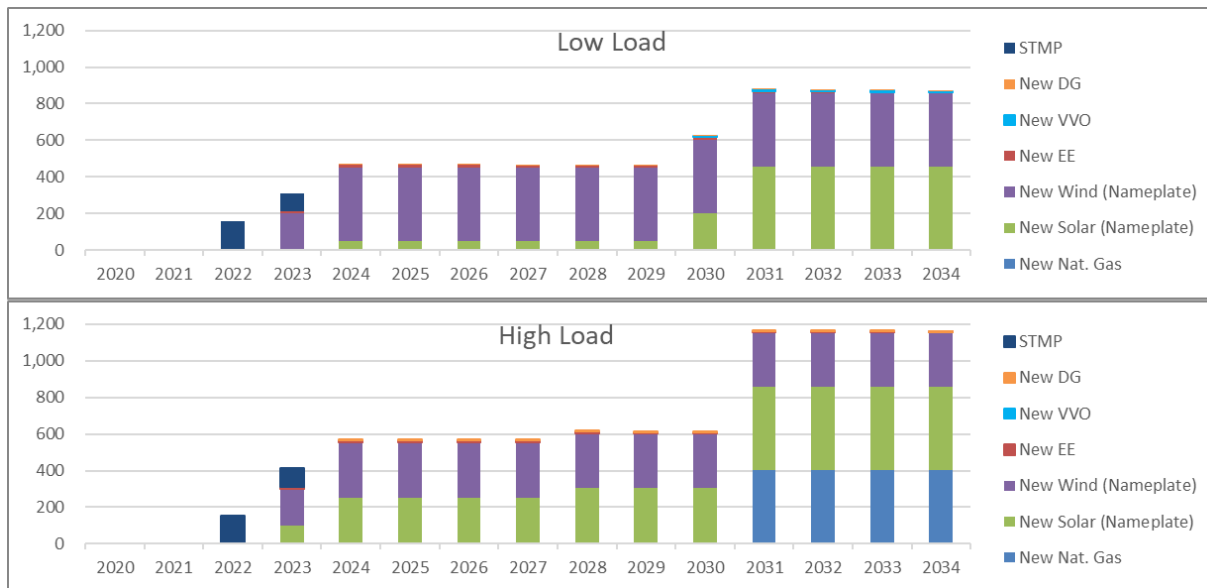
Figure 34. Cumulative PJM Capacity (Nameplate) Additions (MW) for Low Load and High Load Sensitivity Scenarios
