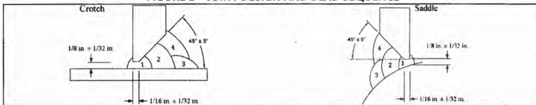
FIGURE 1 – JOINT DESIGN AND BEAD SEQUENCE
