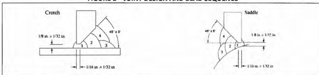
FIGURE 1 – JOINT DESIGN AND BEAD SEQUENCE
