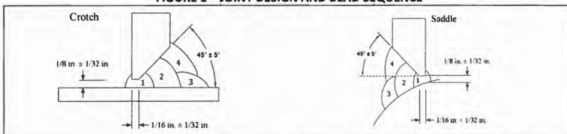
FIGURE 1 – JOINT DESIGN AND BEAD SEQUENCE
