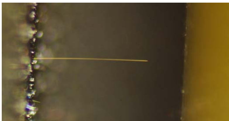
Figure 8 – Whisker Growing between Relay Base (left) and Coil (right) (Photo courtesy of Kinectrics Inc.)
