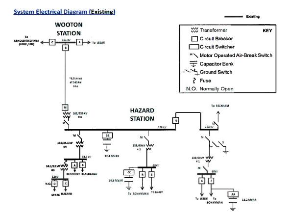
Conversely, the failure of 138 kV circuit breaker N to operate properly in the case of a fault or potential internal fault would produce a complete outage of the Hazard Substation and its elements,<sup>147</sup> along with the loss of service to the customers and 30 MW of load directly served from the Hazard Substation.<sup>148</sup>
