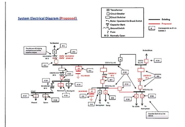
The installation of Project Component 12 allows the new bus-tie 69 kV circuit breaker, the Leslie 69 kV circuit, and Bonnyman 69 kV circuit to be sourced by 138/69 kV transformer #2 when 138/69 transformer # 1 is taken out of service. Likewise, the Daisy 69 kV circuit and the Bonnyman 69 kV circuit sourced by 138/69 kV transformer # 2 can be served by 138/69 kV
