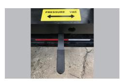
**REVERSE PRESSURE.** Reverse pressure to offload liquids and dislodge debris in hose.
