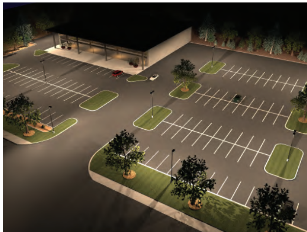
USSL G-A02 LED 14 Fixtures = 2,002 Total watts
