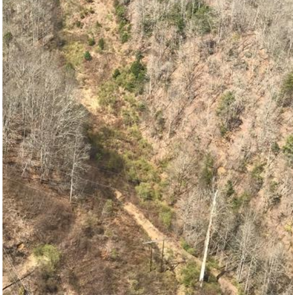
Figure 2. Example of Vegetation Conditions on a Circuit Observed During 2018 Aerial Workload Suvery that has not been Recently Maintained.
