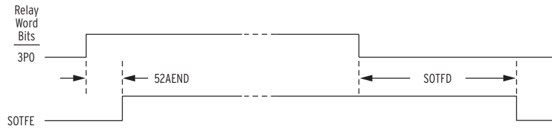
Figure 5.8 SOTF Logic Output (52AEND ≠ OFF)
