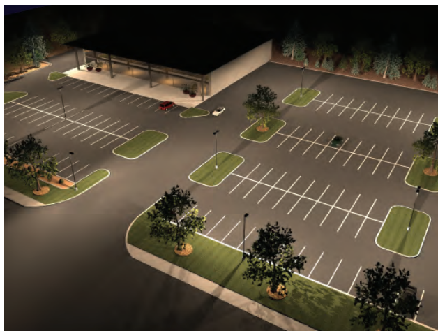
USSSL G-A02 LED 14 Fixtures = 2,002 Total watts
