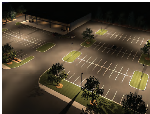
400W Pulse Start Metal Halide 14 Fixtures = 6,370 Total watts
