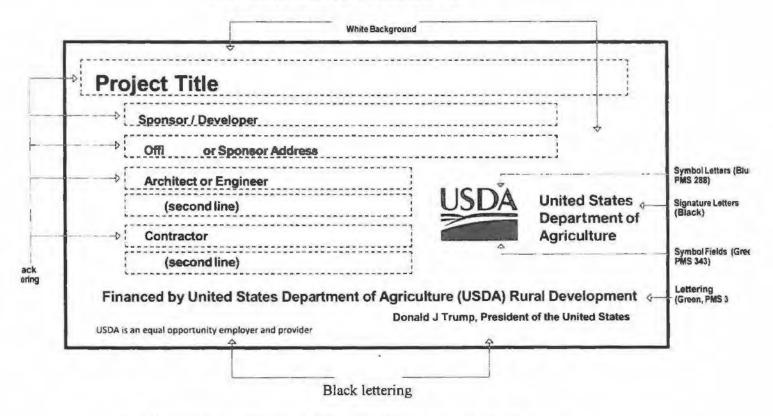
Sign Dimensions: 1200 mm x 2400 mm x 19 mm (approx. 4' x 8' x <sup>3</sup>/<sub>4</sub>") PLYWOOD PANEL (APA RATED A-B GRADE-EXTERIOR)
