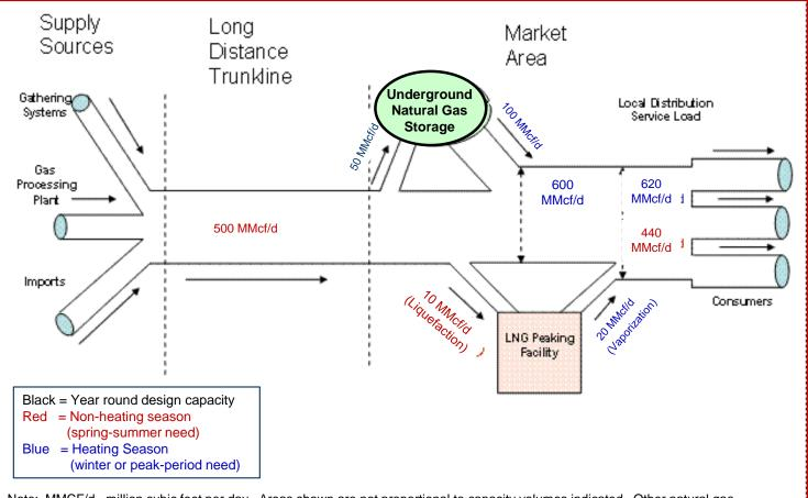
Note: MMCF/d= million cubic feet per day. Areas shown are not proportional to capacity volumes indicated. Other natural gas transmission pipelines may interconnect with and supplement the supplies of the mainline transmission or local distribution company in the market area to meet peak period demands.
