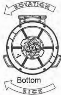
Fig. A – Proper impeller rotation, three phase models
