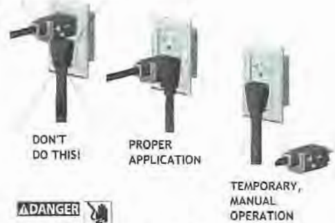
PIGGY BACK PLUG INSTALLATION
