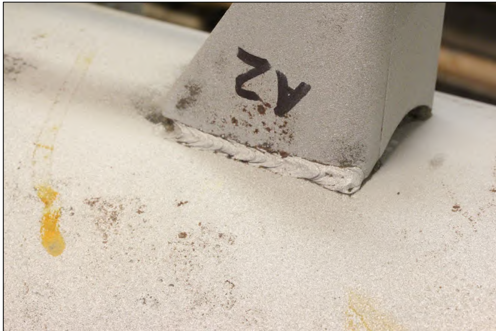
Figure 7. Image of the Lug A2 exterior top weld which exhibited substantial fusion along with undercutting.
