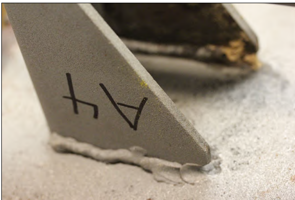
Figure 6. Image of the Lug A4 exterior bottom weld which exhibited substantial fusion except for some overlap and undercut.
