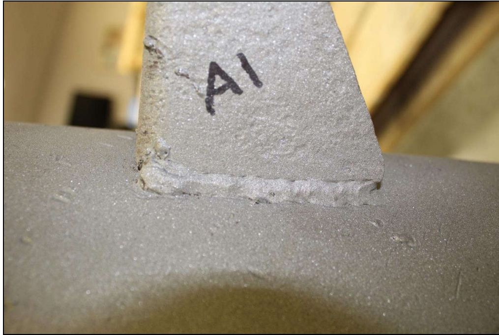
Figure 5. Image of the Lug A1 exterior top weld which exhibited substantial fusion except for some undercut, spatter, and arc strikes.
