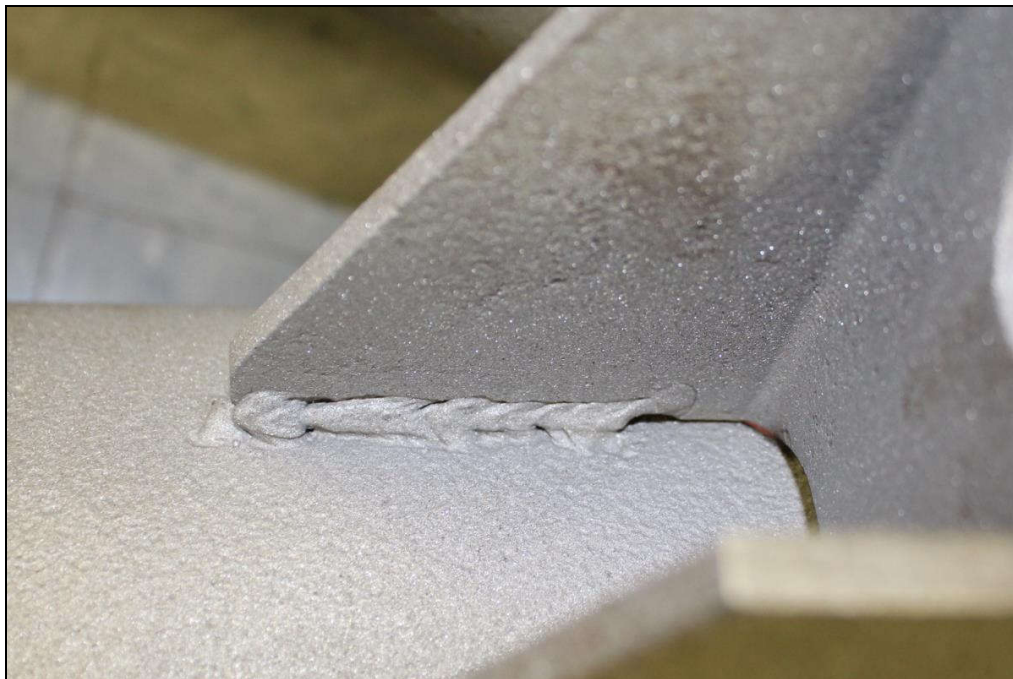
Figure 8. Image of the Lug B1 interior bottom weld which exhibited substantial fusion except for some undercut and arc strikes.
