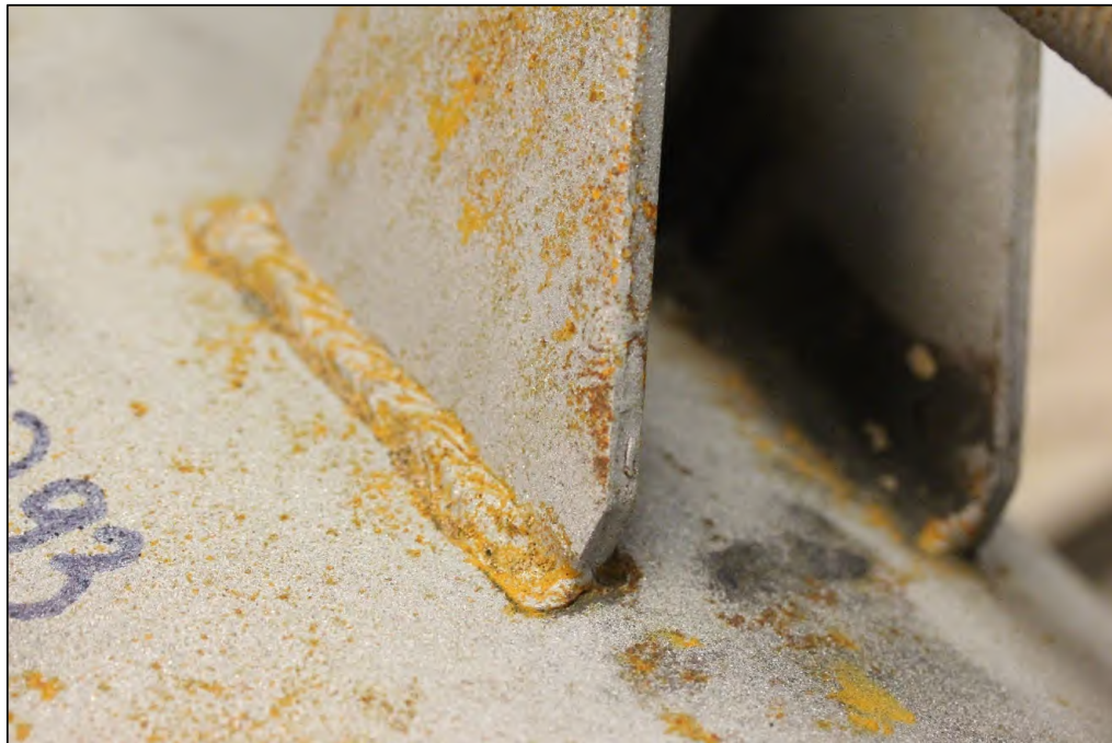
Figure 5. Image of the Lug A1 exterior bottom weld which exhibited substantial fusion except for some undercut, spatter, and arc strikes.
