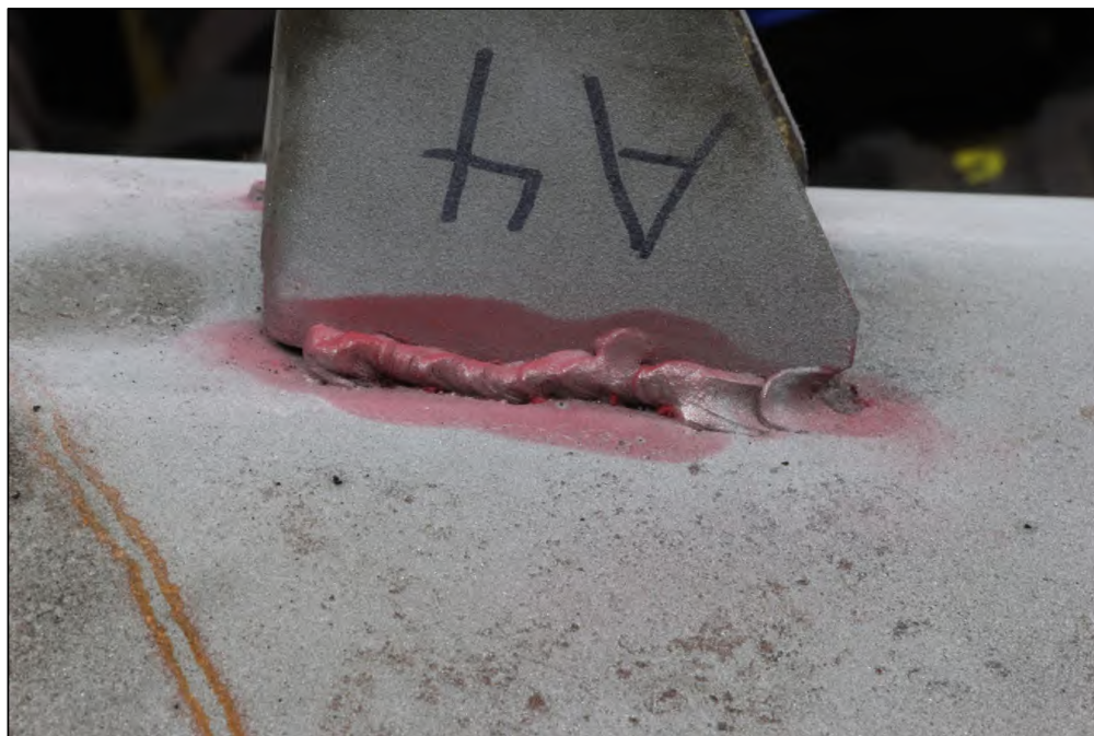
Figure 11. Image of the Lug A4 exterior top weld after dye penetrant media had been used during inspection.
