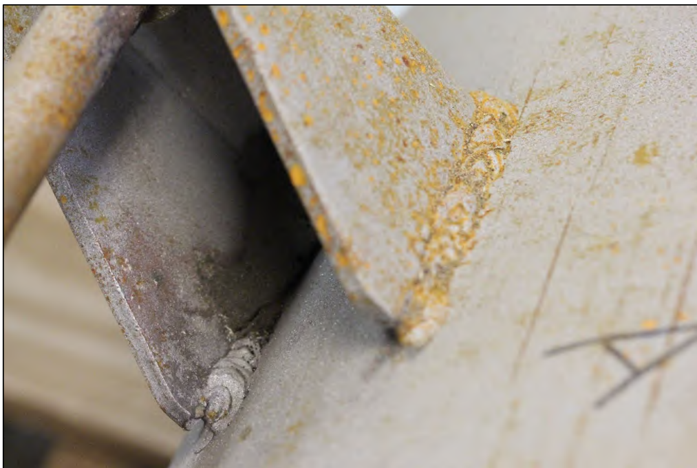
Figure 7. Image of the Lug A4 exterior and interior welds which exhibited general fusions along with undercut, spatter, and overlap.
