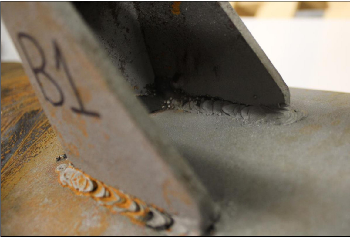
Figure 9. Image of the Lug B1 interior bottom weld which exhibited substantial fusion except for some spatter.
