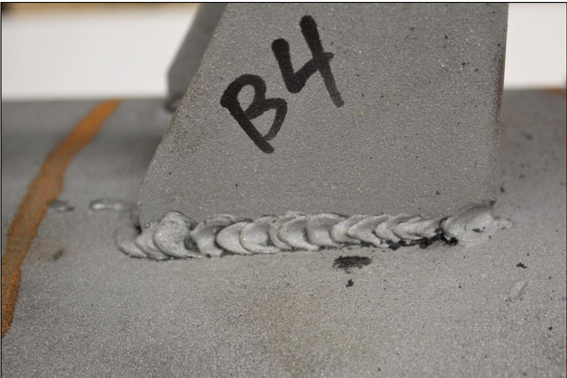
Figure 10. Image of the Lug B4 exterior top weld which exhibited substantial fusion except for arc strikes, undercut, and spatter.
