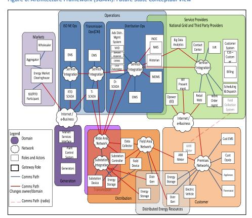
Figure 6: Architecture Framework (SGAM): Future State Conceptual View
