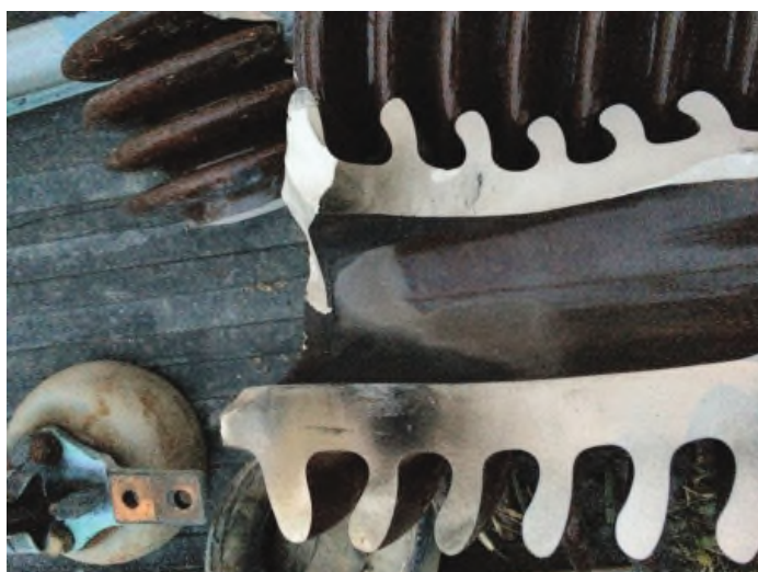
Figure 38: Hollow post insulator after failure.
