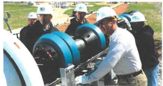
As the "Smart Pig" moves through the pipelines, it collects data on the integrity of the pipeline walls—data which will later be analyzed to pinpoint potential concerns.
