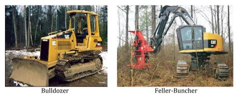
Figure 6. Specialized Equipment Commonly Used in Transmission ROW Clearing and Widening.
