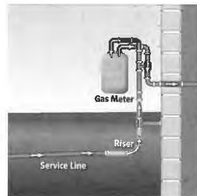
The service riser is a piping component of the natural gas service line that protects the plastic gas service pipe as it transitions from below ground to above ground and from plastic to steel just upstream of LG&E's gas meter.
