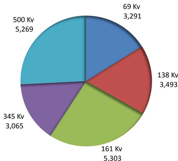
**Figure 3.** Linear Distance of Edge Tree Maintenance per Mile by Voltage Classification<sup>11</sup>.
