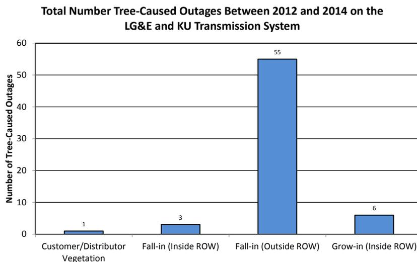
**Figure 1.** Total number tree-caused outages by secondary caused.
