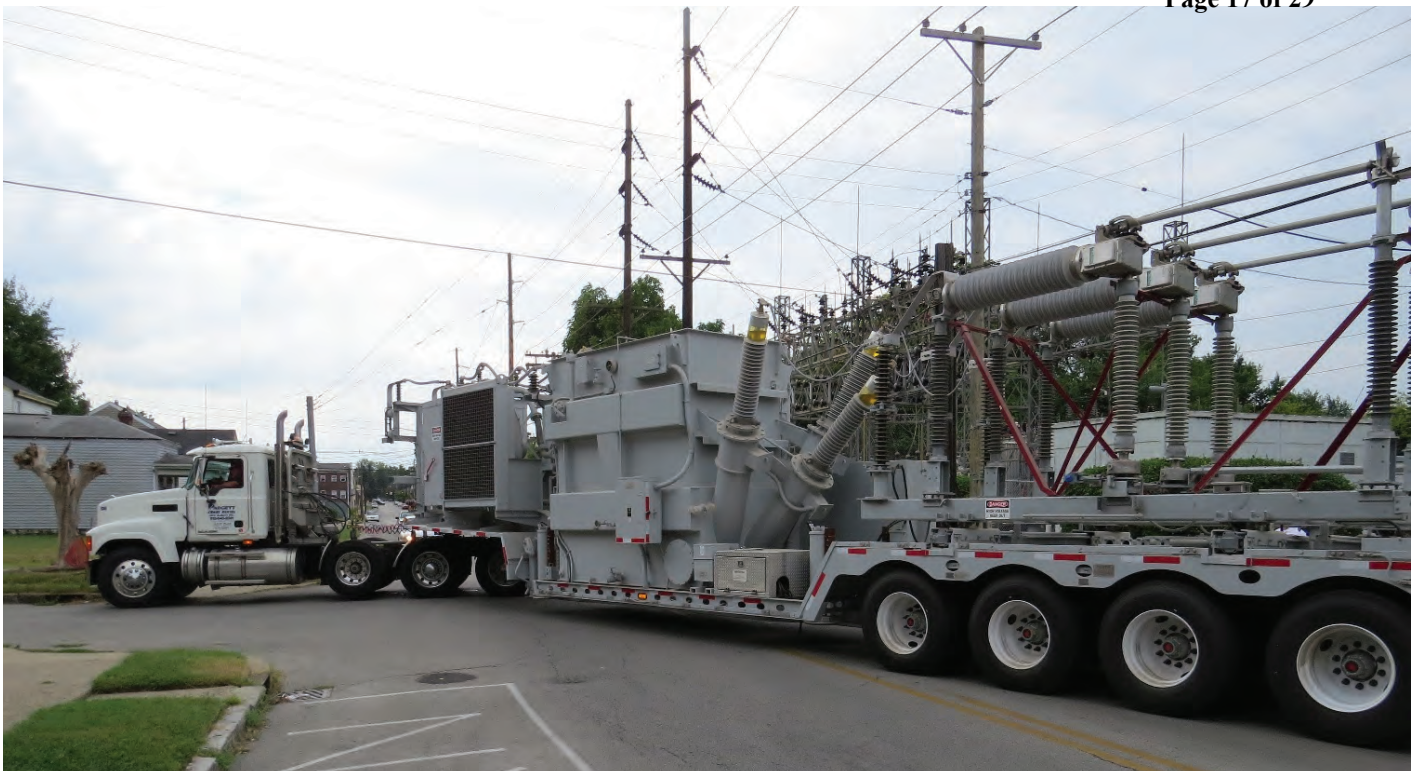
Figure 14: Mobile Transformer owned by LG&E and KU.
