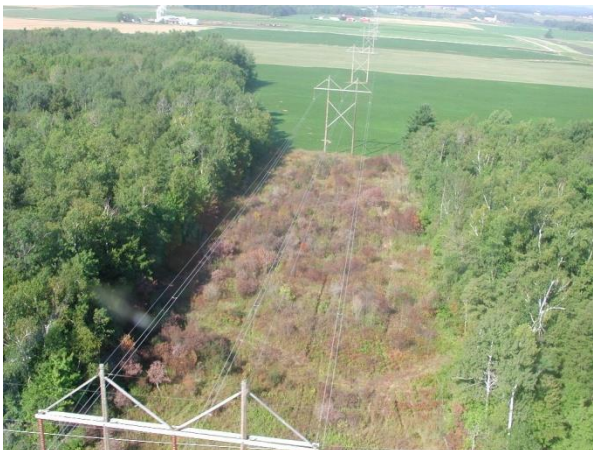
Figure 9. Example of good brush control through the use of herbicides.
