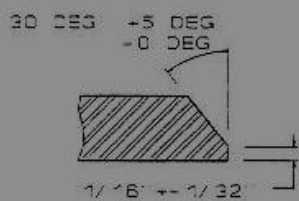
Fig. 1 Standard End Prep. for API Pipe
