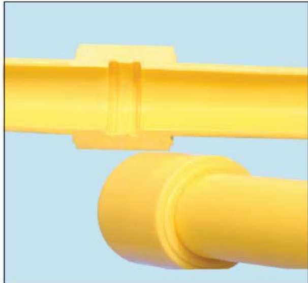
Proper alignment and stab depth. Melt bead flattened due to cold ring. No gaps or voids.
