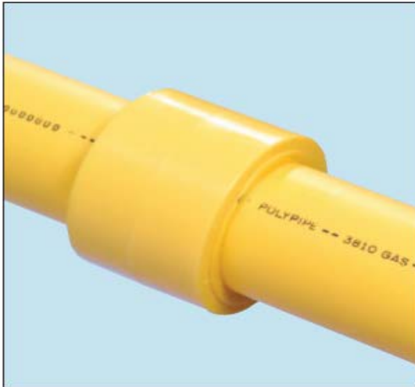
Proper alignment and stab depth. Melt bead flattened due to cold ring. No gaps or voids.
