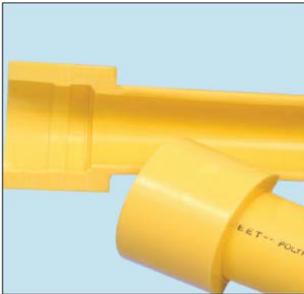
Short stab depth caused by failure to use a depth gauge.
