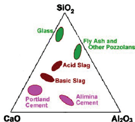
Figure 3.8: Ternary diagram of binders (Douglas and Malhotra, 1987)
