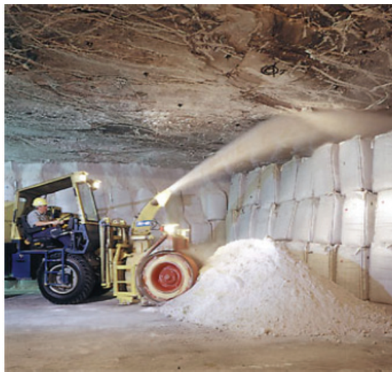
Figure 2.6: Representation of a mechanical backfill (K+S, 2005)
