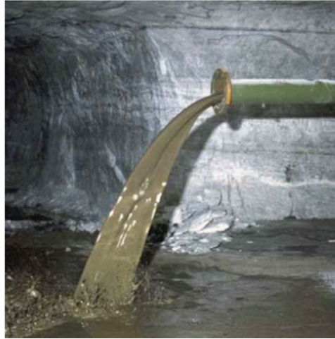
Figure 2.8: Hydraulic backfill (K+S, 2005)
