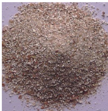
Figure 3.25: Tailing from potash mine Thailand
