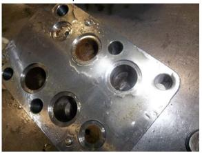
Spool and trip valve showing oxidation as well as varnishing.
