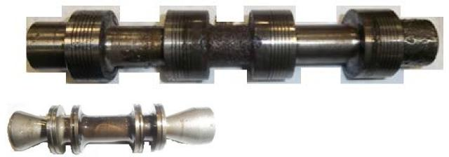
Spool and trip valve showing oxidation as well as varnishing.
