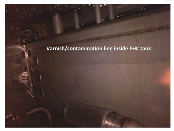
Trip Block assembly was removed from the EHC skid and shipped to Rexroth in Pennsylvania. Rexroth disassembled cleaned and is inspected the Emergency Trip Device/Master trip Solenoid Block. Photos below provided by Rexroth show water, varnish and oxidation. Some components were found in a stuck or sluggish condition. The trip valves were reported to not be functioning at all. Rexroth recommended removal of valve actuators for inspection.
