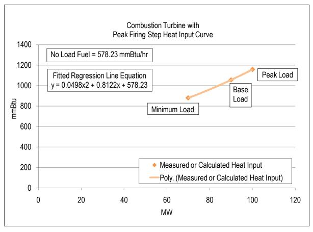
Each diamond in the graph above is a design heat input data point obtained from the original equipment manufacturer or calculated by heat balance. A regression analysis can be performed on the design data to obtain the unit's Heat Input curve as a function of Output with natural gas as a fuel:
