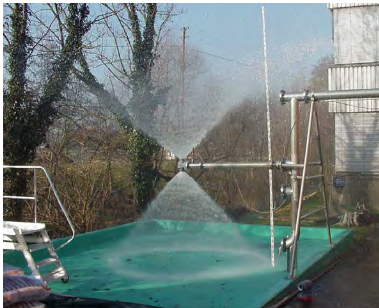
Figure 16. Bi-directional Spray Nozzle Testing
