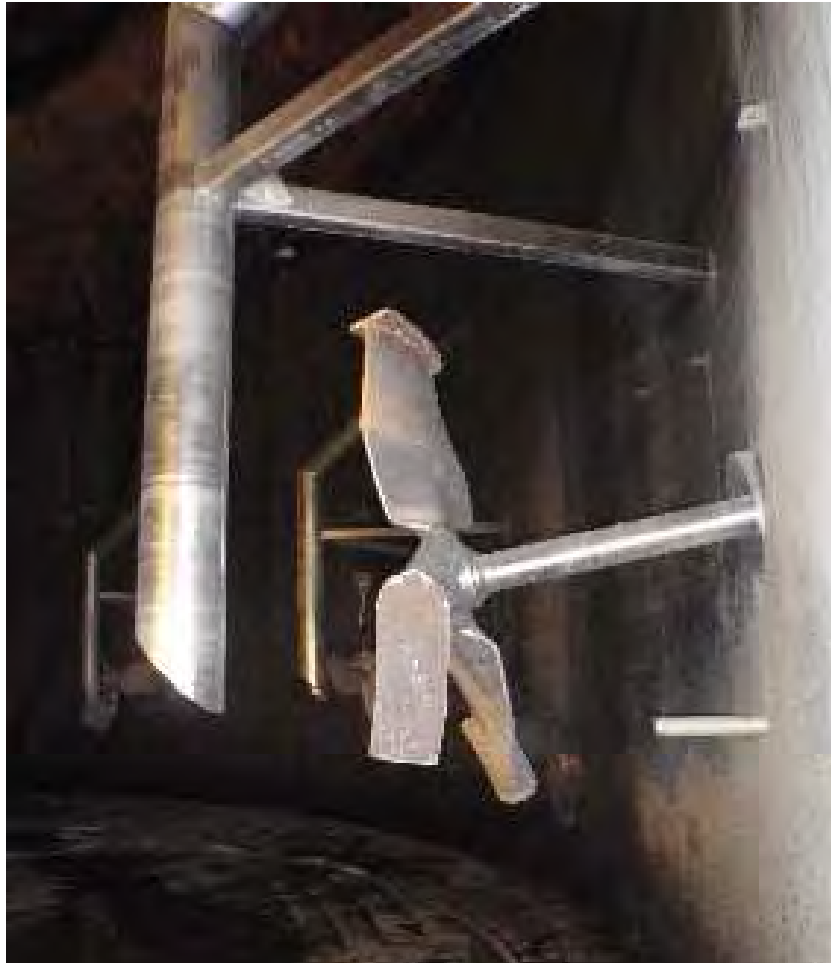
Figure 21: Oxidation Air Lances and Agitator Impellers in Tile-Line Tank
