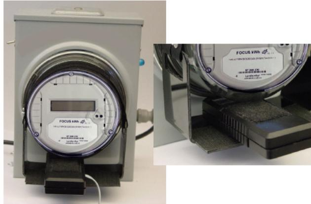
**Figure 2. TS2 FOCUS Endpoint with Universal Opto Wand Holder and Programming Station**
