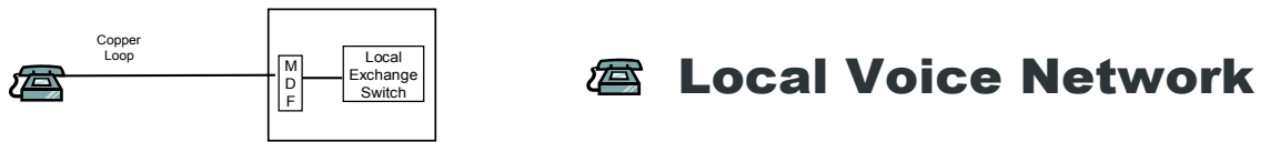
(1) All-copper outside plant; no digital loop carrier (DLC)
