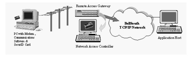
Figure 207 In-Dial Connection Process and Components
