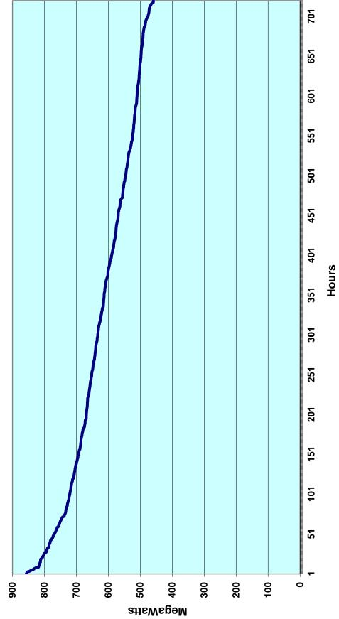
Kentucky Power Company July 2023 Load Duration Curve (Internal Load)
