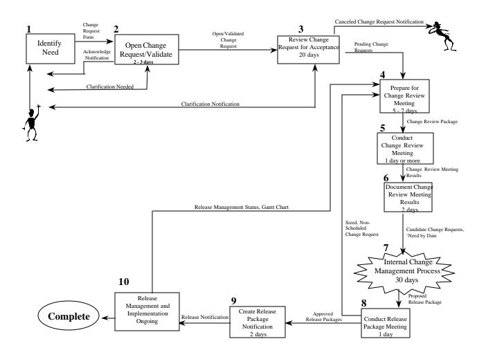
Figure 4-3. Change Control Process Flow
