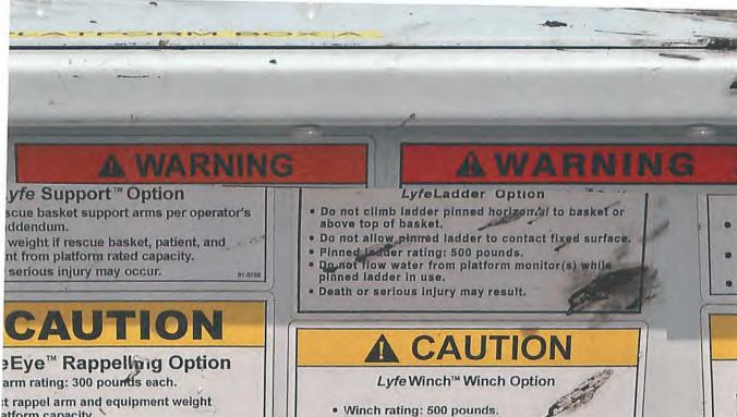
Subtract winch weight from pletform capacity.
