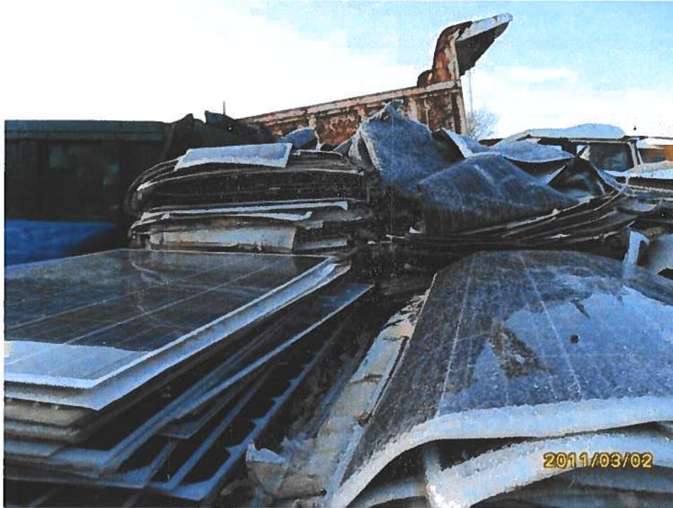
Figure 4: The mangled PV panels in this picture illustrate the nature of broken solar panels; the glass cracks but the panel is still in one piece. Image Source: [http://img.alibaba.com/photo/115259576/broken\\_solar\\_panel.jpg](http://img.alibaba.com/photo/115259576/broken_solar_panel.jpg)
