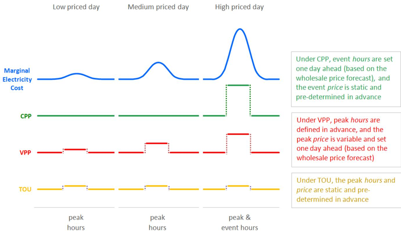
**Figure 1. Time-based rate designs**
