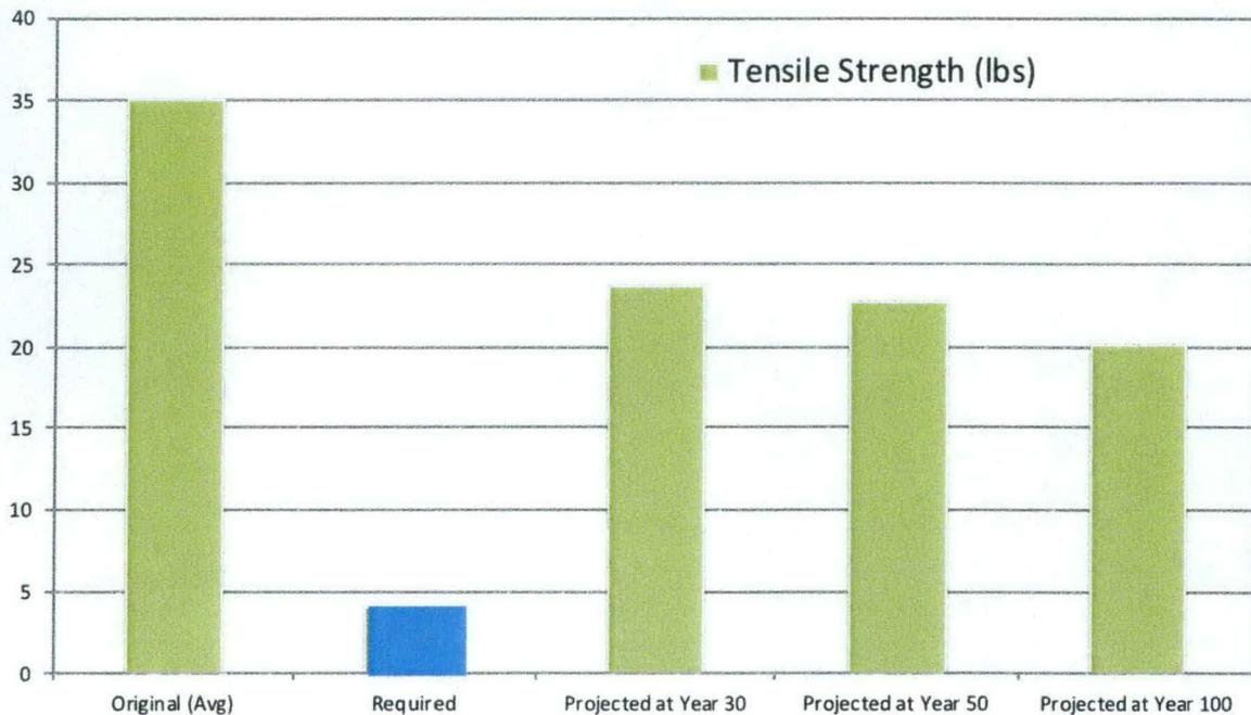
**Figure 2. ClosureTurf® Fiber Tensile Strength**
