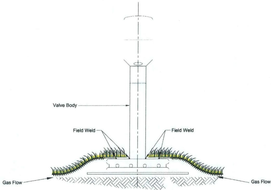
Figure 19: **ClosureTurf®** Passive Gas Vent
