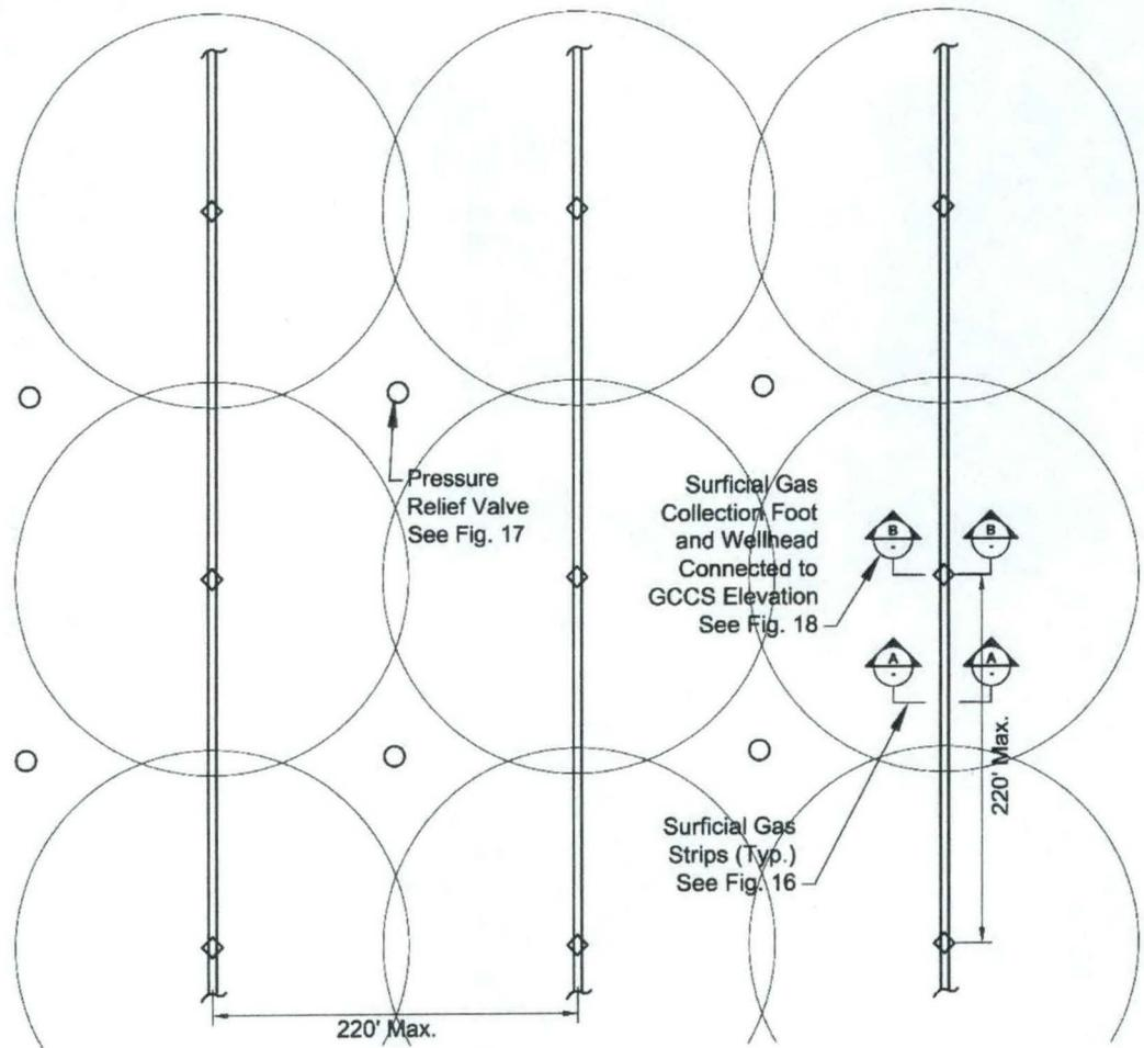
Figure 15: Typical Surficial Collection Strip Placement
