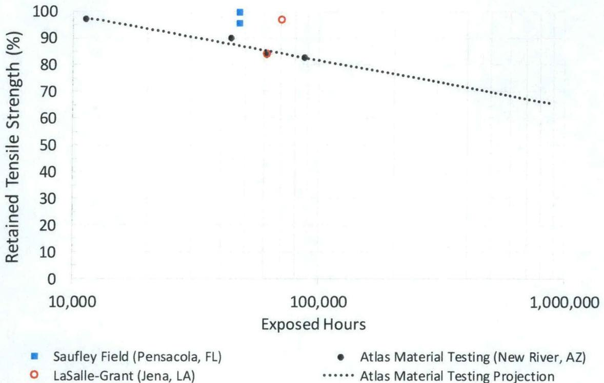
**Figure 3. ClosureTurf® Fiber Tensile Strength, Field Performance**
