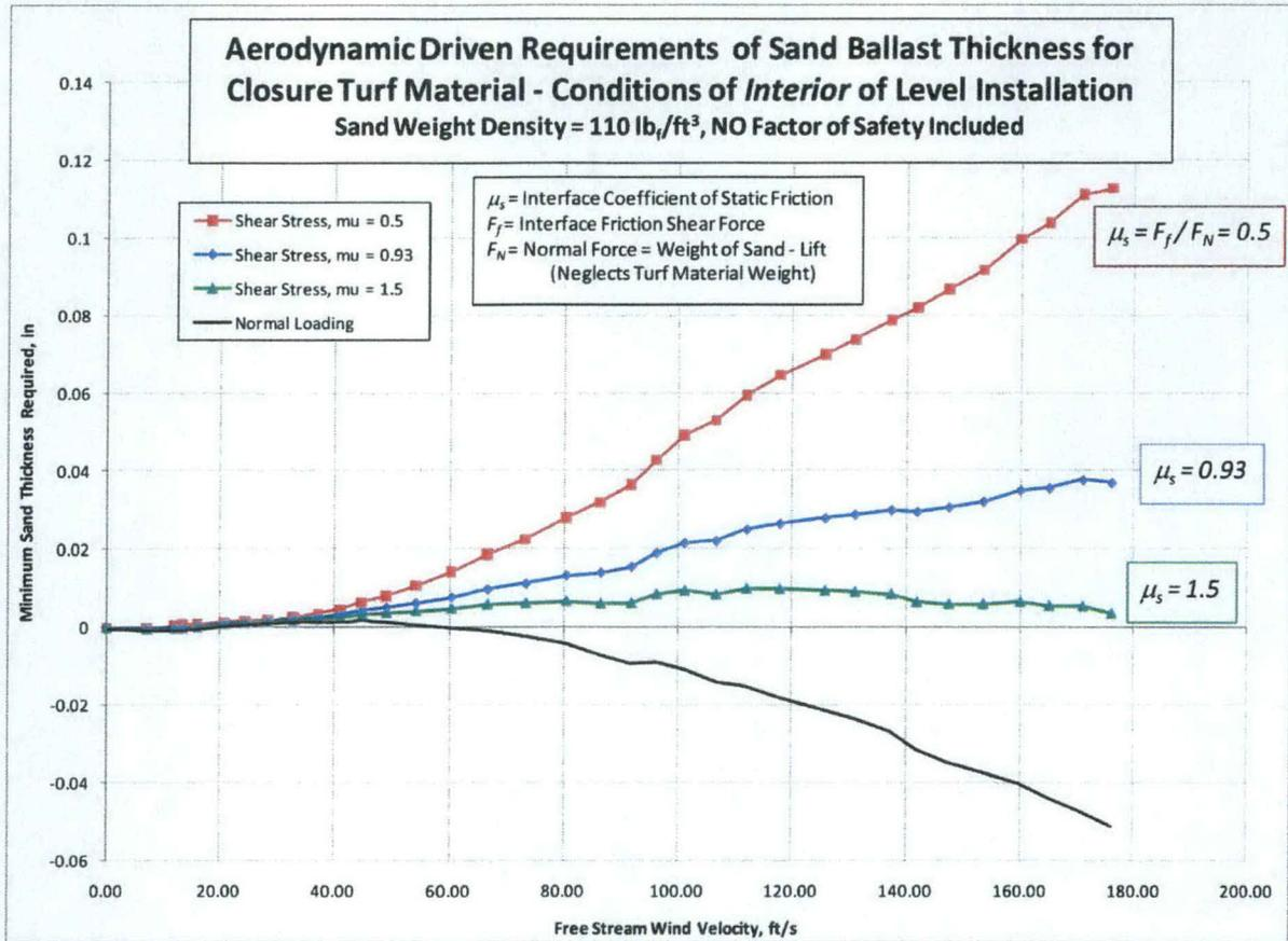
Figure 13: Minimum Sand Ballast Requirement in the Interior of Engineered Turf Installation
