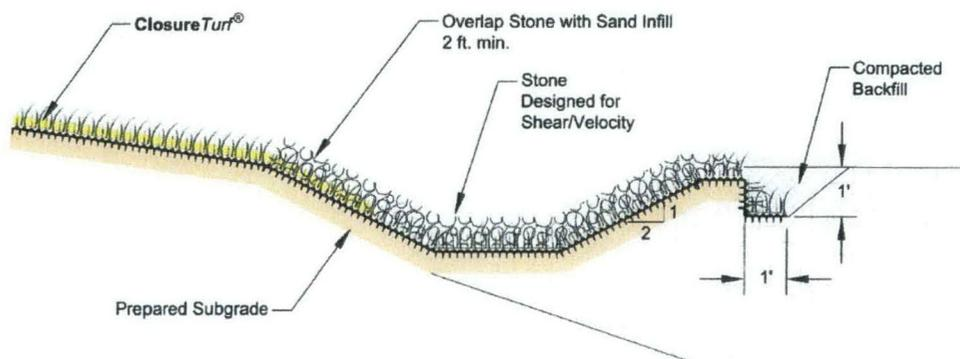
Figure 7: Typical **ClosureTurf®** with Stone Infilled Ditch
