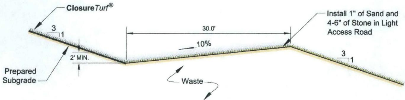
Figure 4: Light Vehicle Access Road Section
