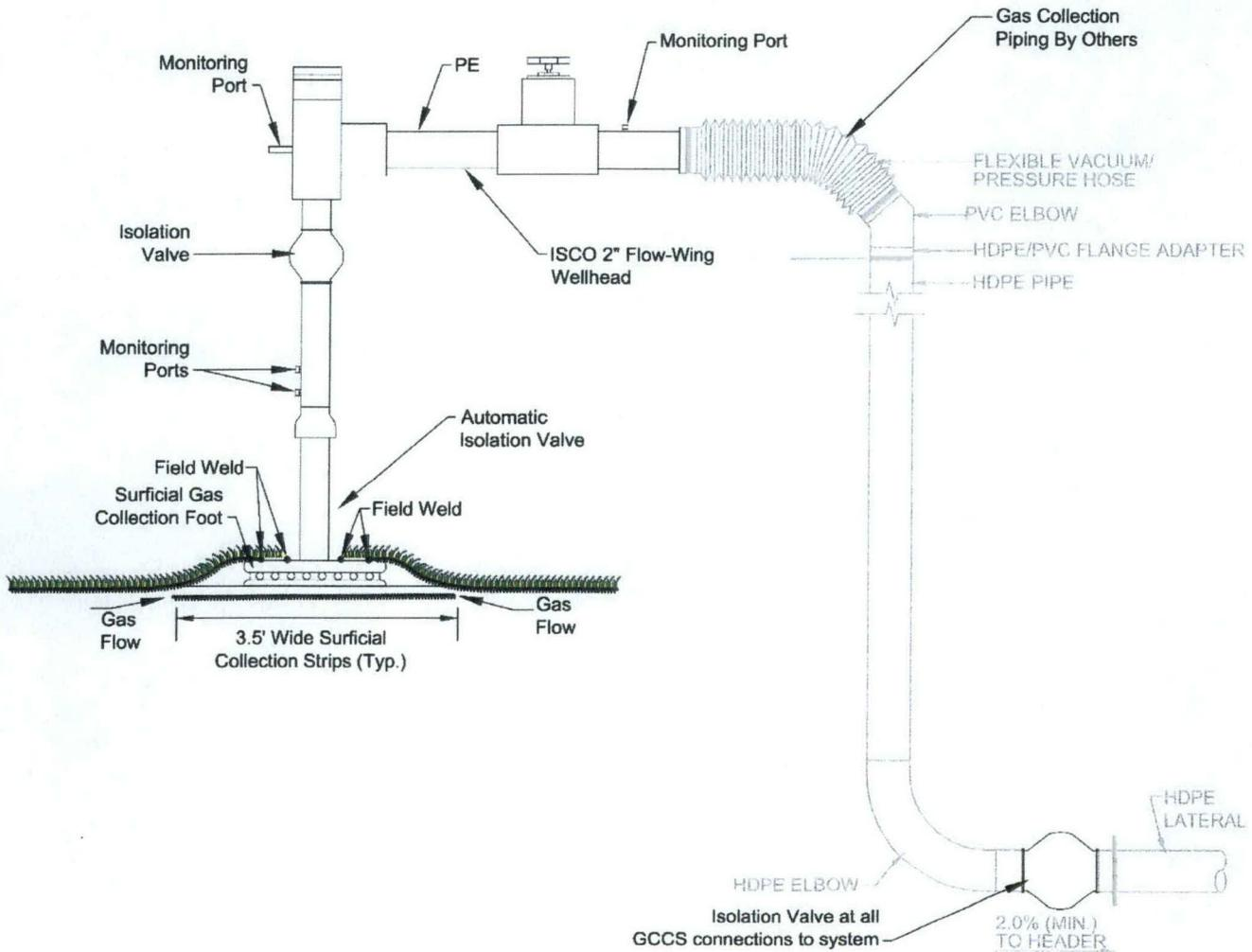
Figure 18: ClosureTurf® Surficial Collection Foot Connection to GCCS System
