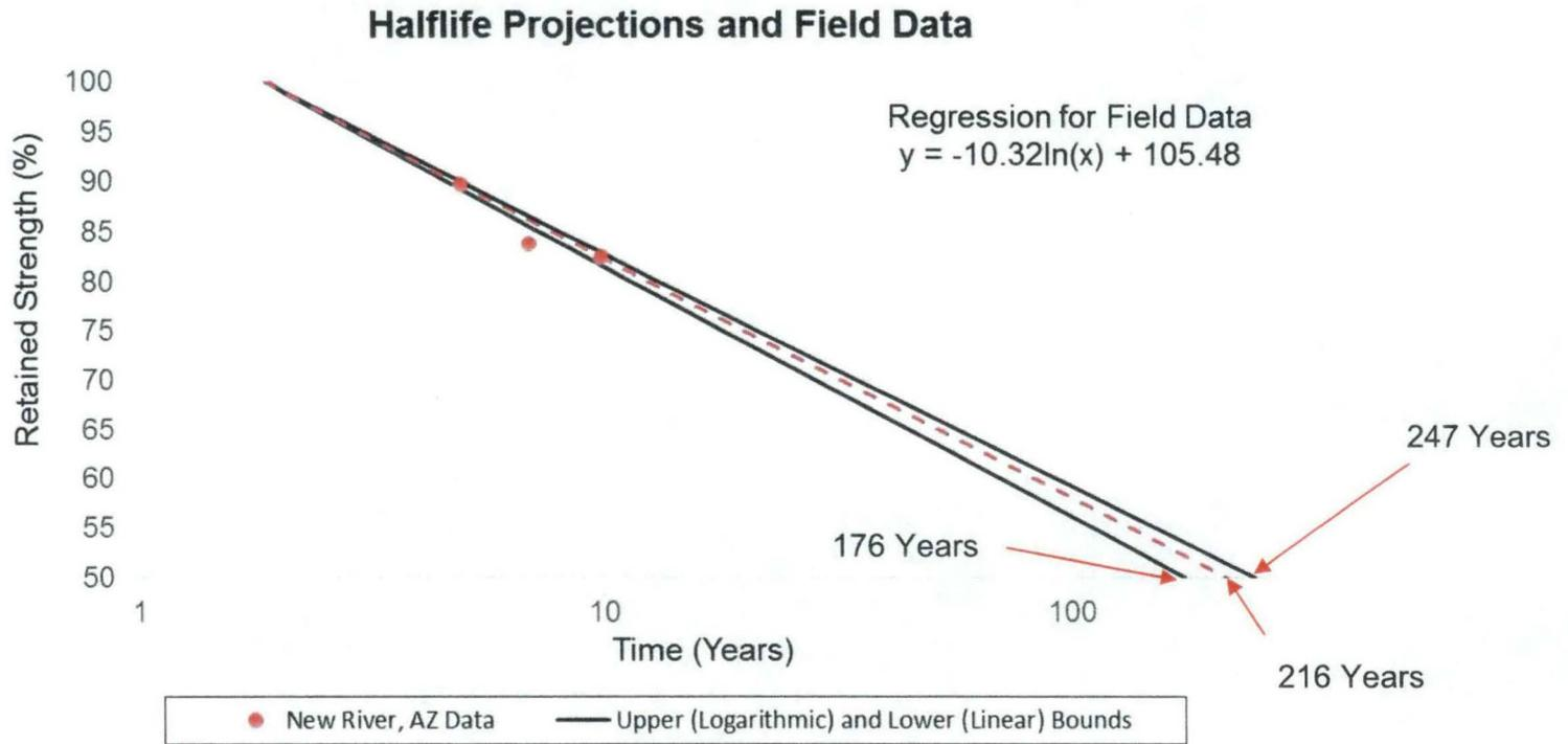
Note: Geosyntec calculated an upper bound half-life of 277 years and a lower bound half-life of 214 years using the same data and method. Difference between Geosyntec and Richgels calculations are attributed to rounding.
