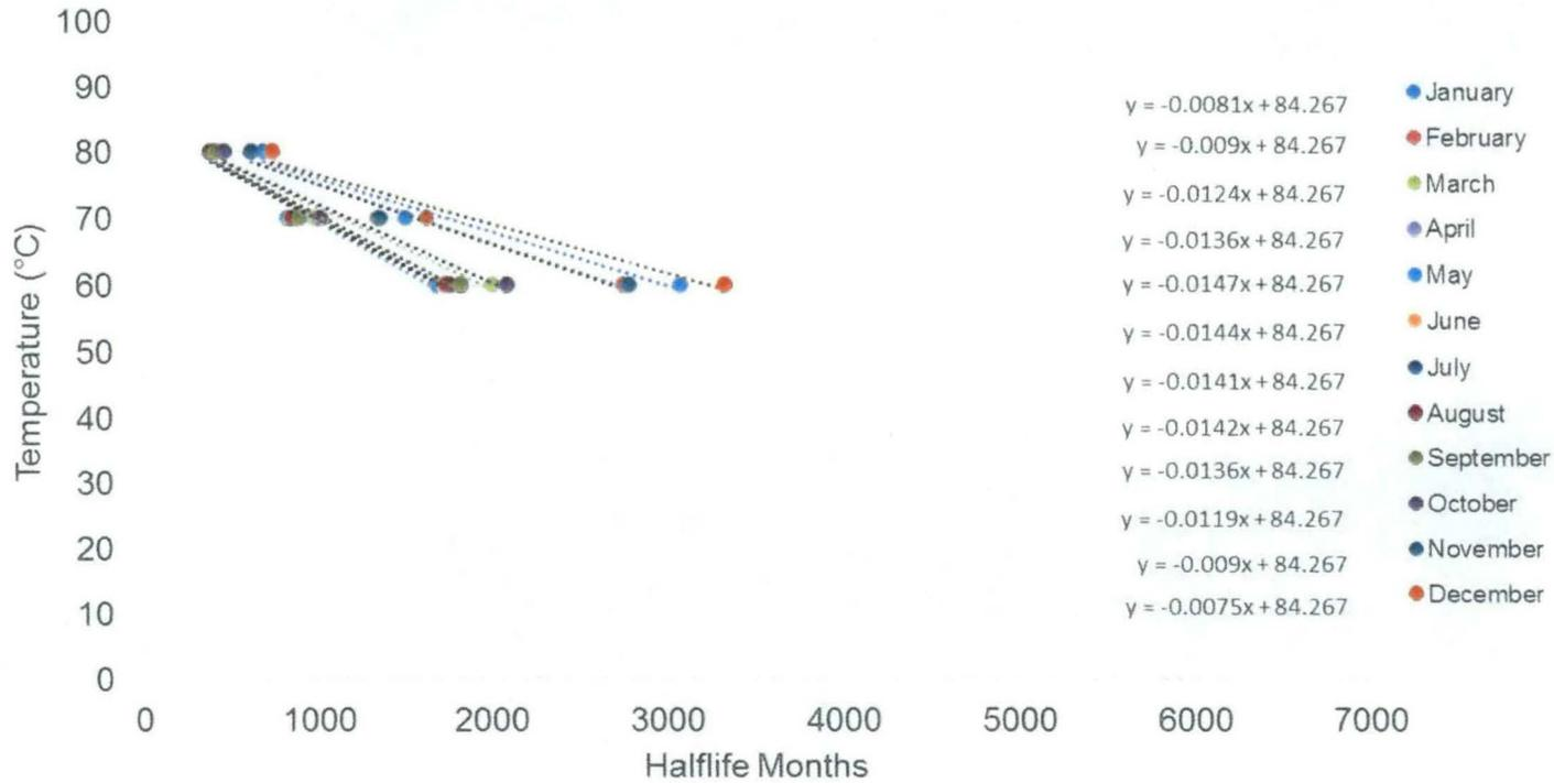
Note: Each month was projected down to the peak turf temperature given in Table 3 to get the half-life months. The inverse of half-life months is half-life loss per month. The sum of all the half-life losses for each month in a year is the yearly half-life loss, the inverse of which is the half-life.
