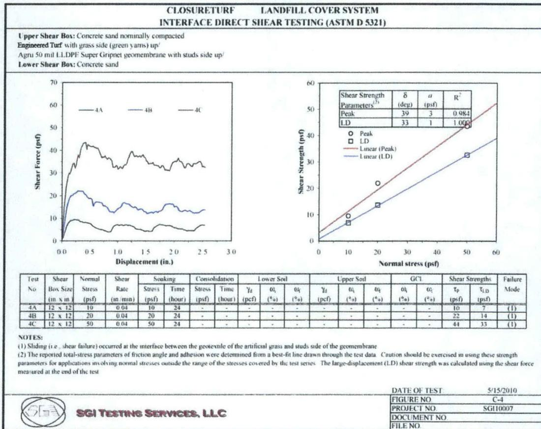
Figure 10: Interface Direct Shear with Low Normal Stress at 10, 20 and 50 (psf). Engineered Turf and Agri 50 mil LLDPE Super Gripnet®.
