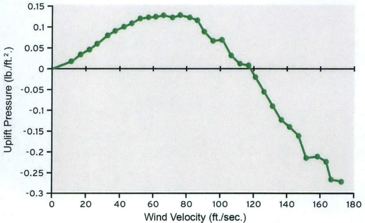
Figure 11: Georgia Tech Research Institute Wind Tunnel Chart Uplift Pressure vs. Wind Velocity
