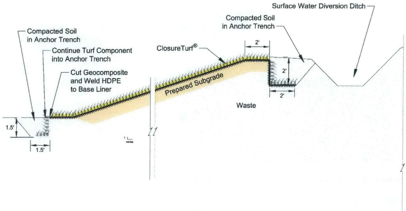
Figure 6: Typical **ClosureTurf®** Anchor Trenches at Top and Bottom of Slope
