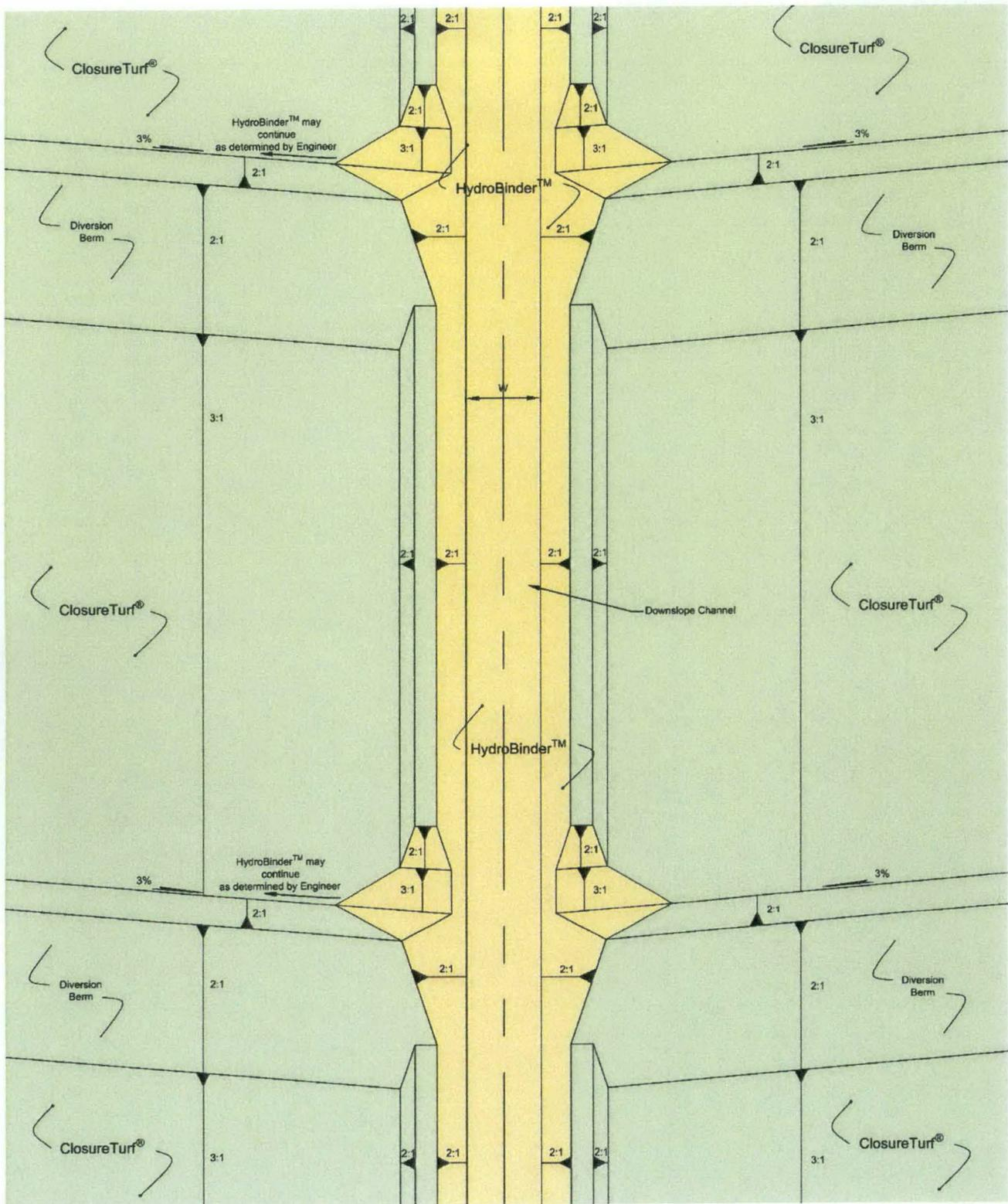
Figure 9: Typical **HydroBinder®** Infill Placement in Downslope Channels
