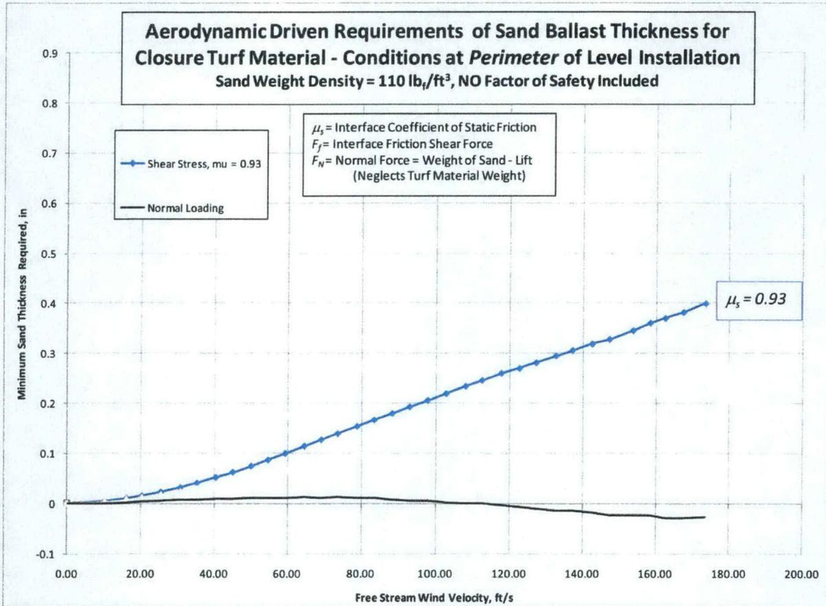
Figure 12: Sand Ballast Minimum Requirement at the Perimeter of Engineered Turf Installation
