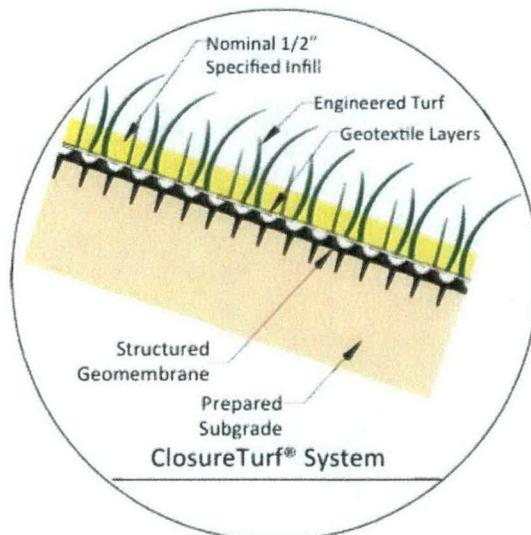
**Figure 1. ClosureTurf® Cross-Section**
