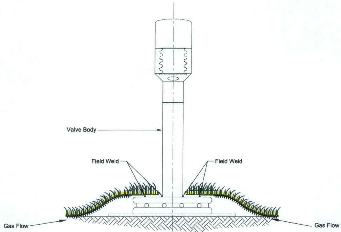
Figure 17: **ClosureTurf®** PE Pressure Relief Valve (Patent Pending)
