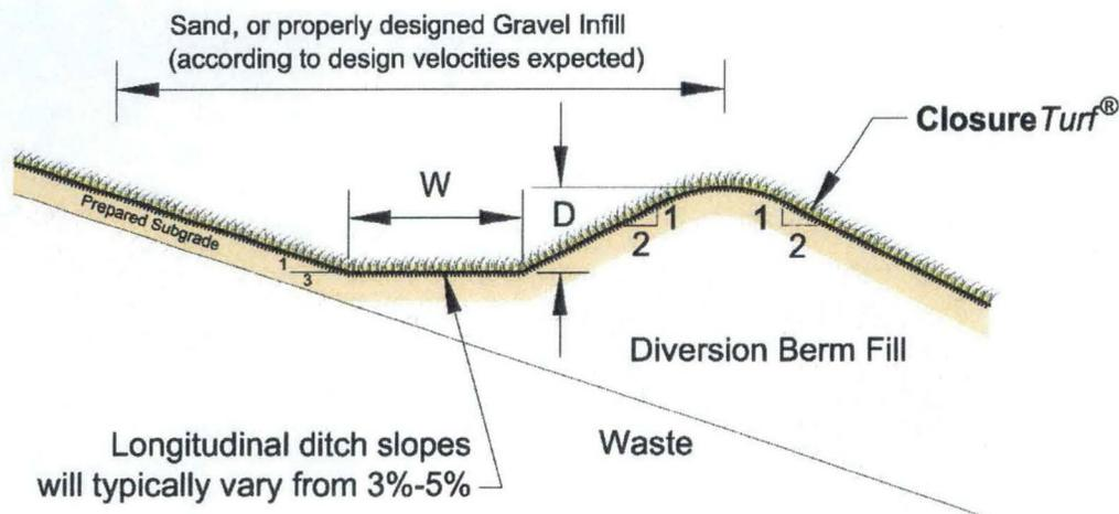
Figure 3: Typical Diversion Berm
