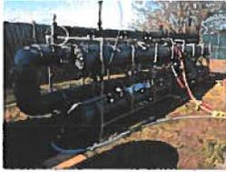
PeroxyChem's Disinfection Pilot Reactor (DPR) enables side-stream testing to measure effectiveness at different dose rates under varying effluent quality conditions.
