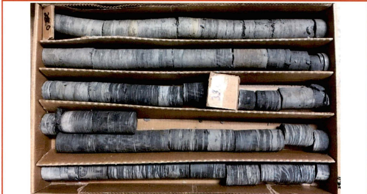
PHOTO #2 – Rock core sample at B-1 from about 28 to 38 feet below existing grade (bottom of the core at lower right corner)
