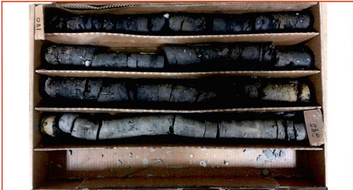
PHOTO #1 – Rock core sample at B-1 from about 18 to 28 feet below existing grade (top of the core at upper left corner)
