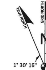
BASED ON KENTUCKY STATE PLANE SINGLE ZONE AND DETERMINED BY GPS OBSERVATIONS COMPLETED ON MARCH 12, 2019
