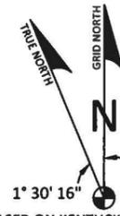
BASED ON KENTUCKY STATE PLANE SINGLE ZONE AND DETERMINED BY GPS OBSERVATIONS COMPLETED ON MARCH 12, 2019
