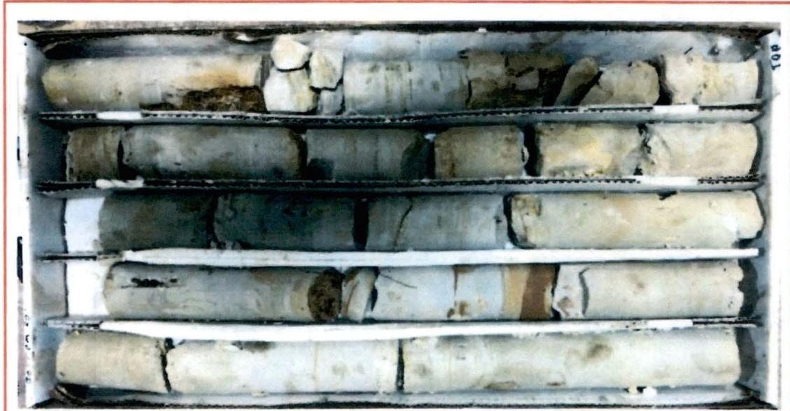
**PHOTO #1 – Rock core sample at B-1 from about 10 to 20 feet below existing grade
