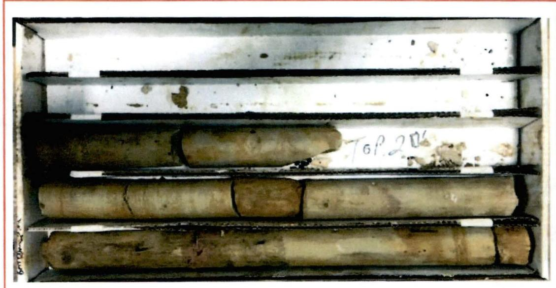
**PHOTO #2 – Rock core sample at B-1 from about 20 to 25 feet below existing grade
