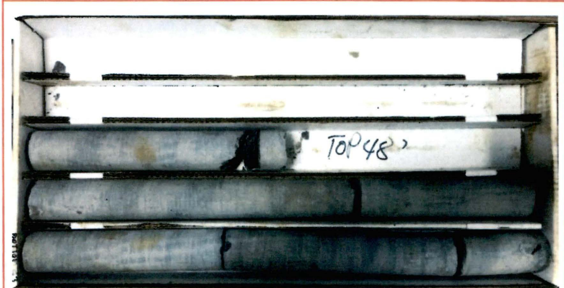
PHOTO #1 – Rock core sample at B-1 from about 38 to 48 feet below existing grade (top of the core at upper right corner)
